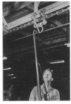
and trailers are hooked onto the conveyor by telescopic masts.
