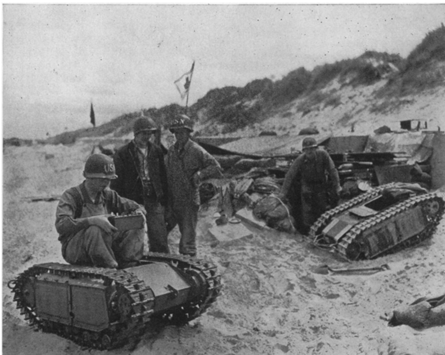
NAZI "BEETLE" —United States Navy men take apart an Axis miniature tank loaded with explosives—to see what makes it tick. First used at Anzio, the robot vehicles are sent forward against Allied lines with a mechanism by which they can be exploded at a distance. Allied marksmen in most cases have picked off the "beetles" while they were still too distant to do any damage.
