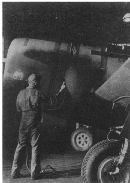
"LIQUID ENVELOPE" — A P-47 Thunderbolt gets a spray of hard skin which will protect it against wind and weather during its ocean voyage.
