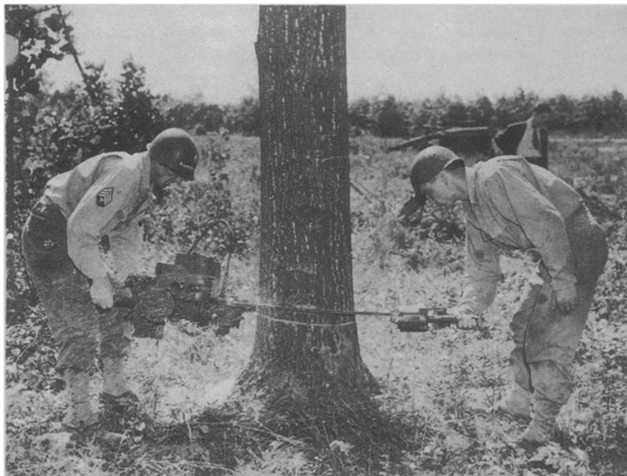
CHAIN SAW —Powered by a motor similar to the type used to propel out-board motor boats, the chain saw weighs about 100 pounds, and is so well balanced that it can be operated in any position. All operations are controlled by the operator on the left.
