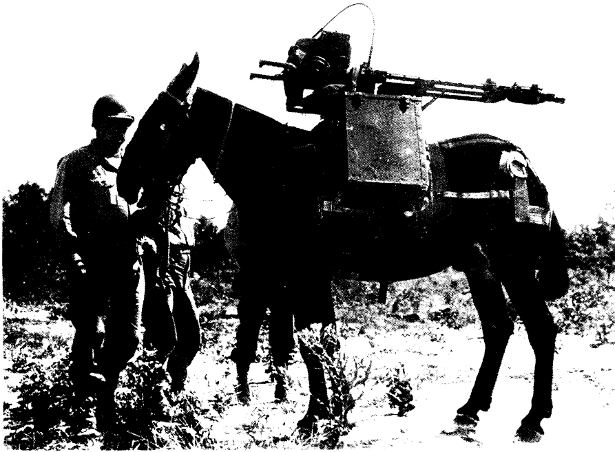
G. I. MULE —He is carrying a chain saw which will cut through a tree or hard wood log 12 inches thick in twelve seconds. Photographs by Fremont Davis, Science Service Staff photographer.
