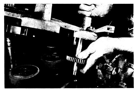
OUTWEARS RUBBER—Originally developed to prevent gear breakage in the event of jamming, a unique type of power transmission involving rubber rings that mesh with metal gears on revolving turret machinery was in use in the plant of a large radio manufacturer, before the rubber shortage. In the course of the rubber conservation program, it was found that when the rings were made of compar, a vinyl resin derivative compounded by Resistoflex Corporation, their service-life was increased five times.
