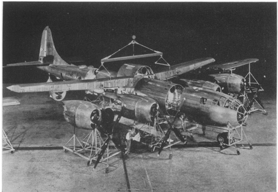
ASSEMBLY OF THE B-29 —This "exploded" view of the B-29 Superfortress shows graphically the system of production in which major units of the giant airplane are brought together in the final assembly stages. This makes final assemblage a matter of joining and connecting. Visible in the fuselage section at center of main wings is part of the tunnel used by crew members in passing over bomb bays between fore and aft pressurized cabins of the airplane.
