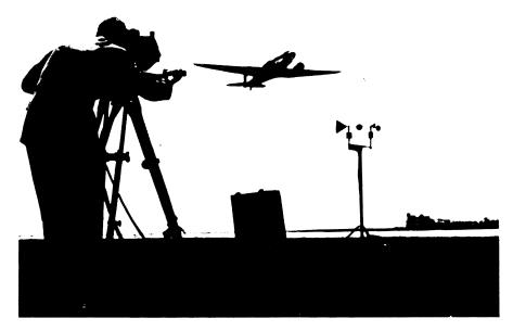
ADDS TO AIR SAFETY—This camera system provides a scientific method of determining the required runway lengths by recording and analyzing take-off and landing characteristics of airplanes (See SNL, Nov. 18, p. 325). In actual practice, the wind indicator unit would be located near the runway, while the camera would be located 1500 feet away from the runway.
