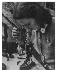
measured to a millionth of an inch by embedding them in a plastic block which is then carefully cut so that the ends of the wire show on the surface. The picture shows the block being examined under a powerful microscope with micrometer eyepiece.
