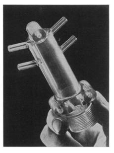
KEEPS WATER OUT—To guard against the possibility of water in 100 octane gasoline, Douglas Aircraft employs this alternate static vent drain of transparent Tenite plastic in the fuel system of one of its planes. If any water should be present in the gasoline, it is automatically drained to this vent, where it accumulates and regardless of altitude, never freezes.
