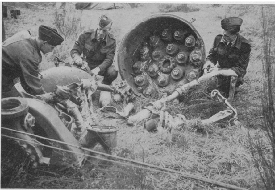
JETS EXPOSED —The 18 jets through which the propellant mixture in the V-2 rocket is sprayed into the combustion chamber are shown here. These RAF pictures (see also cover and facing page) were made of a rocket which fell in Belgium.
