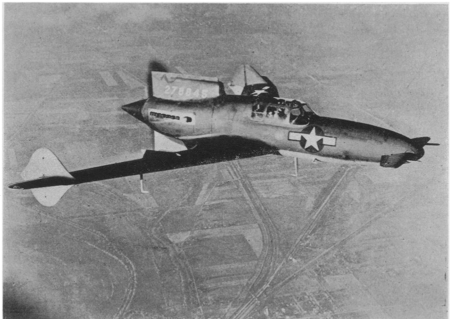
"ASCENDER" —This XP-55, a cross between a flying bomb and a long-necked goose, flies better than it looks. Tailless, its elevator controls are in the nose, and the rudder control is on the sweptback wing tips. Powered by the Allison 1710 engine, from the ground the plane appears to be flying backwards. Official U. S. Army Air Forces photograph.
