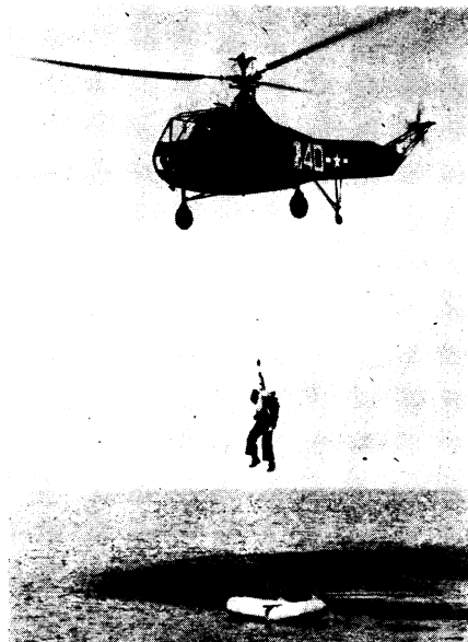
HYDRAULIC HOIST —This is the method used in a helicopter air-sea rescue system. It consists of a pump and motor each about the size of a man's hand—which was found capable of lifting and controlling a 400-pound load at two and one-half feet a second. Official U. S. Coast Guard photograph.
