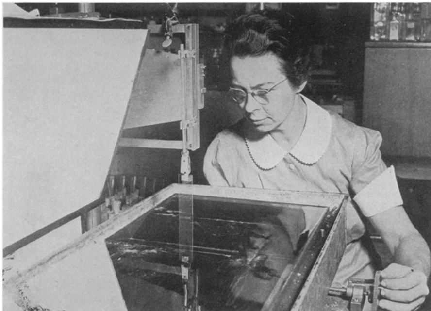
"BUILT-UP" FILM —Dr. Blodgett, working in her laboratory at the General Electric Company, is building the thin films, which afford scientists a valuable thickness gauge, by dipping them in and out of the water. The crank in her left hand raises and lowers the glass which holds the film.
