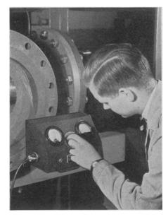
CONTROL UNIT, for a new allmetal thermocouple vacuum gauge, operates directly on 100-volt AC and indicates low pressures accurately and continuously. The light, portable instrument, pictured above, may be carried about and connected to thermocouple gauges in any part of the factory vacuum system.
