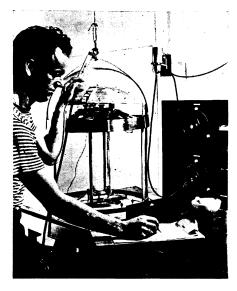
LENSES COATED—Mounted on a rounded panel inside a large bell jar, lenses for naval combat instruments are given a coating of magnesium fluoride in the optical shop at the Mare Island Navy Yard, Vallejo, Calif., to improve their light transmission and field definition characteristics. Jim DeMartini, chemist, is checking the thickness of the coating.
