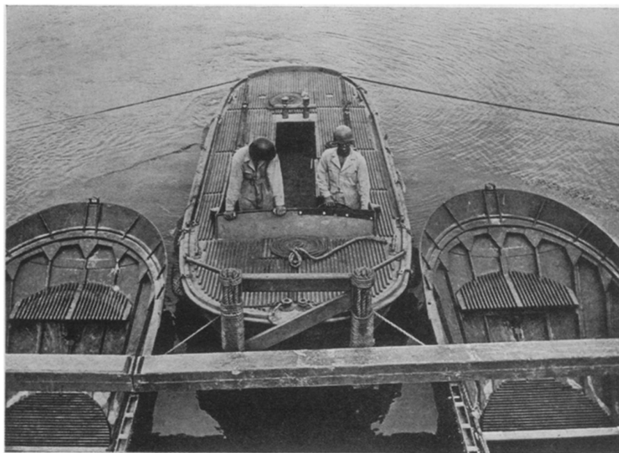
UTILITY POWER BOAT —This new boat, capable of propelling bridge-rafts or ferries with loads up to 80 tons in swift currents, is now being shipped overseas. Each of its two propellers is driven by a gasoline engine capable of developing 80 horse-power at 3,000 revolutions per minute. The maximum pulling power is 4,000 pounds and the top speed is 15 miles per hour. Official U. S. Army photograph.
