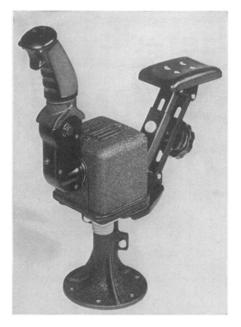
ONE-HAND CONTROL—This new control is used on all present heavy bombardment planes. The position of the stick and arm rest is readily seen to be arranged to give comfort to the pilot.
