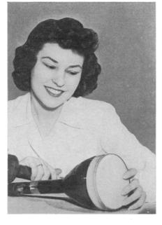
tubes, for large-screen home television, are five inches in diameter, less than half the 12inch prewar tubes on the face of which the picture was read directly. The new tube, shown above, gives a brighter picture and is cheaper to make.
