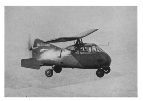
CONTROLLABLE WINGS—Greater safety and easier handling of personal aircraft may result from this new development. The controllable wing eliminates the necessity of ailerons, elevators and rudders.
