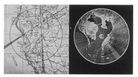
RADAR BOMBSIGHT—At the left is an ordinary air navigator's chart of Tampa Bay, Fla. At the right is the same "target" as seen on the radar bombsight screen. The straight lines across the water near the top of the picture are bridges and causeways. The small white dots show how boats and ships look to the radar eye. Notice how clearly land and water masses are distinguished.
