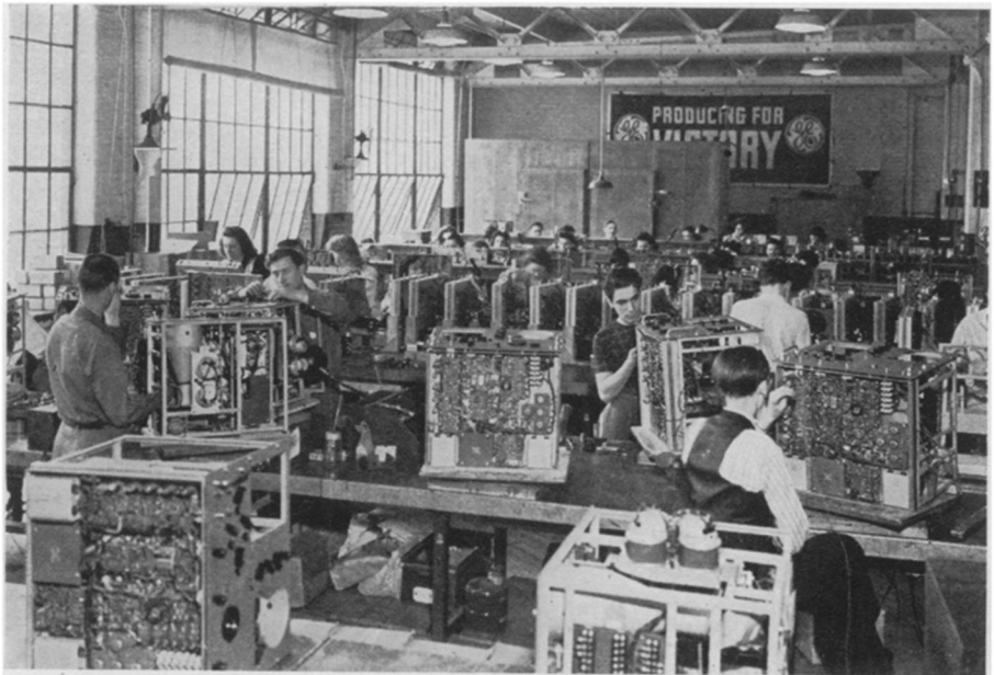
RADAR MANUFACTURE —This is the way those super-secret radar factories looked. Here the equipment is being assembled in a General Electric plant for use in the U. S. Navy. Notice that the large tube which acts as electronic eye for the set is visible in side view in the set being handled by the worker at the left. The face of the tube shows in the set in the left foreground.
