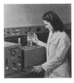
ELECTRONIC DRIER, laboratory model, employs a 100-watt radio-frequency generator to provide heat for drying out liquids placed in a moderate vacuum under the small dome shown in the picture. It is designed for research men working with biological solutions and heat-sensitive chemicals.
