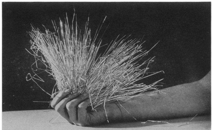
STOPPED RADAR —A handful of the aluminum foil which was scattered in the air to blot out radar echo. Photograph by Fremont Davis, Science Service staff photographer.
