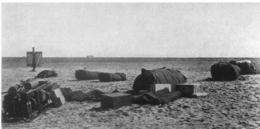
QUICKLY ASSEMBLED —The three sections of the pneumatic LCT packed in their compact bundles prior to inflation.
