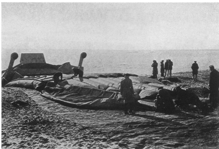
FOOLED THE ENEMY! —Here is a decoy LCT that misled the enemy on Allied ports of embarkation shown being assembled.
