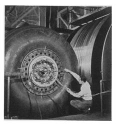
BOMBER TEST—This massive testing machine simulates landing effect of future giant bombers. This three-quarter-ton tire stops the 158 ton steel inertia wheel in 20 seconds. The 110-inch tire is slammed against the steel wheel as the steel speeds around at two miles a minute, simulating actual landing conditions without risking personnel or equipment.
