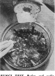
FUNGI TEST—Radar and radio equipment, switchboards, transformers and hundreds of other kinds of apparatus which went into the Pacific war theater in huge quantities were tested against attacks from every type of mold common to Pacific areas. Sixteen different kinds of fungi here receive their weekly meal of homemade bread to keep them robust and destructive. Photograph from Westinghouse.
