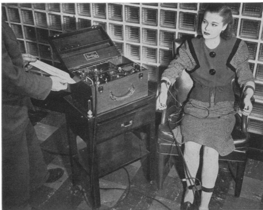
DIRECT RECORDING —This portable electrocardiograph inks its record of heart action directly on paper without photographic darkroom procedures. The inventor, Paul Traugott, president of the Electro-Physical Laboratories, Inc., explained that his cardiotron can be used in the home by the physician if necessary.
