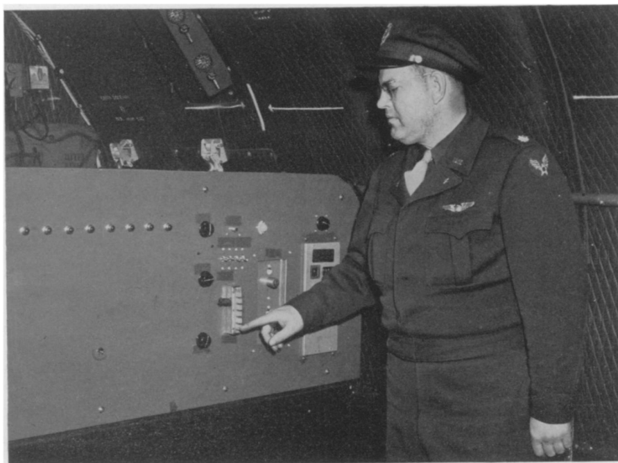
CONTROLS FLIGHT —Push buttons on the Automatic Flight Controller installed in a giant C-54 "Skymaster" cargo plane are explained by Maj. Paul R. Biggers, project engineer on the development of fully automatic flight.
