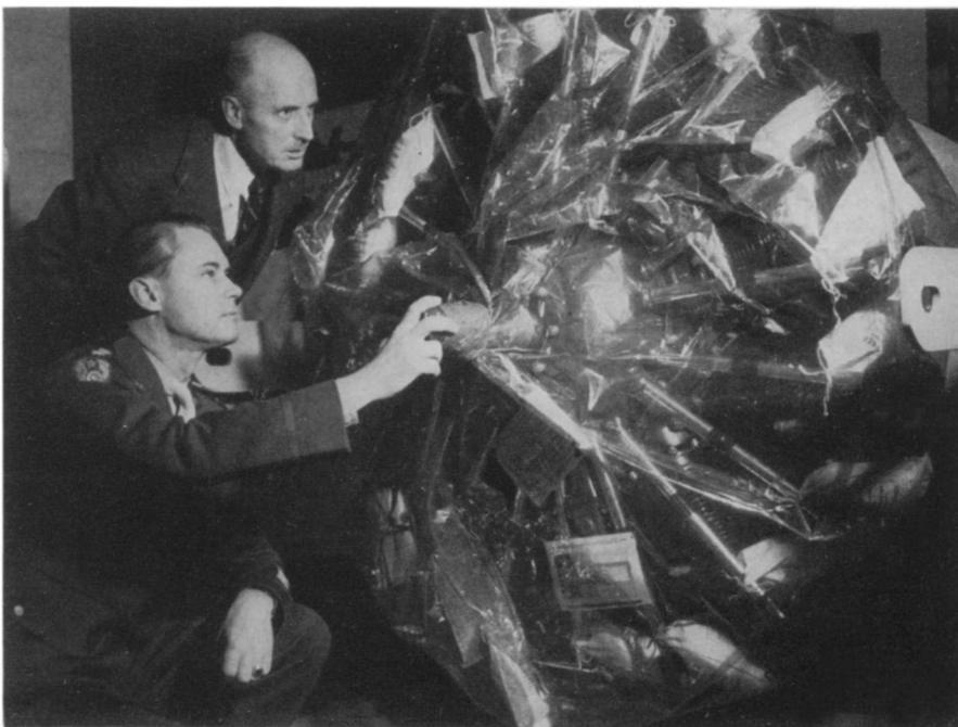
WASP ENGINE PROTECTED —Dr. Henry Butler Allen, secretary and director of the Franklin Institute, explains the protective refinishing of the Wasp No. 1 engine to Lieut. Gen. Hoyt S. Vandenberg. Through the moisture-proof wrapping of pliofilm can be seen the numerous bags of protek-sorb silica gel and (lower center) a humidity indicator.
