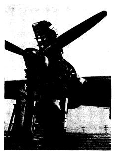
SAVES TIME—Gaping metal jaws frame the 2500 horsepower Wright engine of the Lockheed Constellation as a mechanic makes a minor adjustment. Ground crews who have worked with the new type cowling say that as much as 15 to 20 minutes is saved every time an engine must be serviced or inspected. This saving in time will be passed on to Constellation airline passengers in reduced ground time during scheduled flights.
