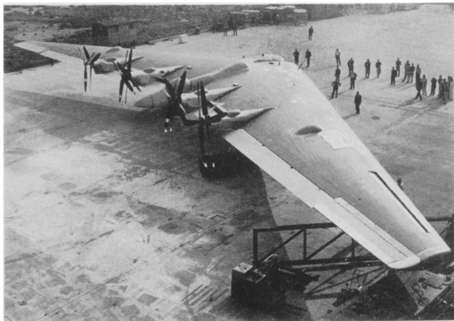
ALL WINGS —Four eight-bladed co-axial propellers, driven by four Pratt and Whitney Wasp Major engines, are expected to push this Northrop Flying Wing XB-35 long-range bomber along at high speed. Wing tip nearest the camera shows one of the wing slots which aid the Flying Wing's efficiency at slow speeds. At high speeds, where the slots are not needed, automatic doors close over them, "streamlining" the smooth surface.
