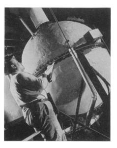
MAKING PERFUME—One of a battery of vacuum stills that isolates from a crude chemical substance, such as coal tar, the usable perfume component is shown at the du Pont plant, New Brunswick, N. J. The fragrance being created here is aubepine, a characteristic odor of hawthorn.
