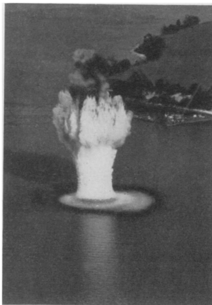
Joint Army-Navy Task Force One Photograph BIKINI REHEARSAL—But this is not an atomic bomb. It is a TNT underwater explosion performed as a preliminary test at the Naval Mine Warfare Test Station, Patuxent River, Md., to provide data for underwater atomic explosions at Bikini Atoll.
