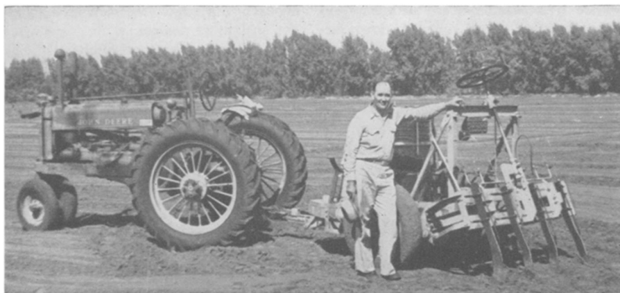
INJECTOR —Applicator of Shell Chemical Corp. used for treating land at Weatherford Farms, Linn, Texas. Photo by R. A. Biron, Dow Chemical Co.
