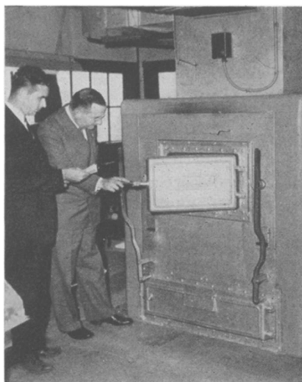
FURNACE —Laboratory model of the new Williamson furnace, with draft system at rear, is being inspected.
