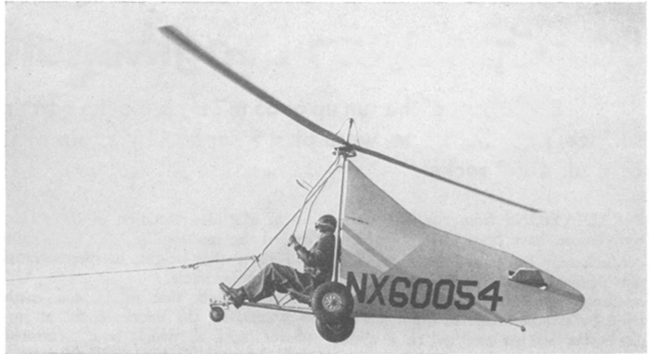
POWERLESS CRAFT —This Gyroglider, without wings or engine, developed by General Electric, is being towed by a jeep.
