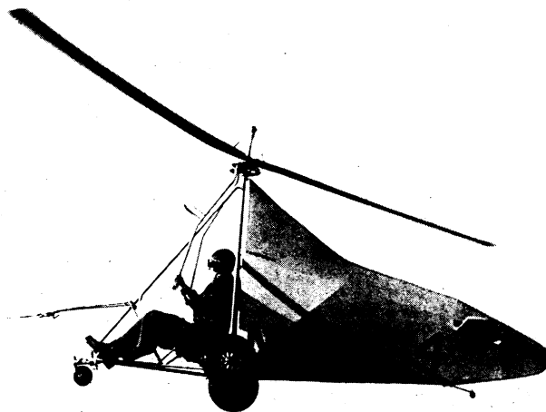
POWERLESS CRAFT —This Gyroglider, without wings or engine, developed by General Electric, is being towed by a jeep.
