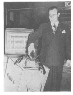
SHIPPING container, refrigerated, has a magnesium cooling unit inside that is operated by gases emanating from dry ice. The box itself, shown in the picture, weighs 20 pounds empty and has an outer wall of vulcanized rubber and a lining of aluminum, with a light insulating material between them.
