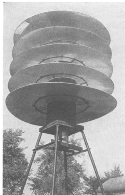
FROST DEFENSE —Machine uses infrared heat to prevent frost damage. It was developed at the Michigan State College Agricultural Experiment Station.
