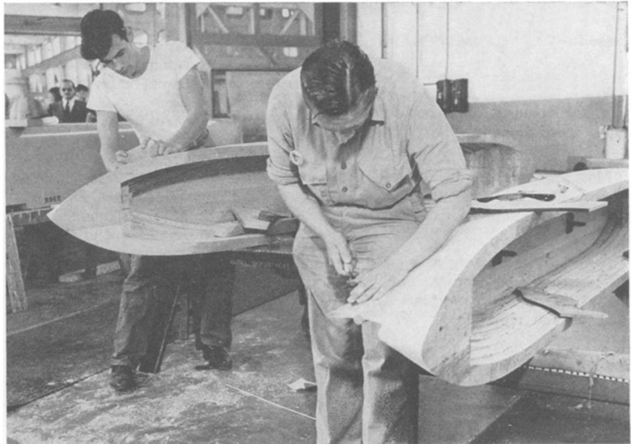
NO INSIDES —Without superstructure, a model ship is hollow and fashioned from layers of Western pine glued together.
