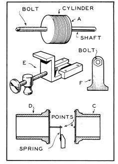
The brass cylinder has spiral grooves cut in it to correspond with the threads of the bolt. The experimenter can cut similar grooves in the cardboard box. A sharp knife or the point of a phonograph needle can be used to scratch the surface, then make deeper the marks by going over the scratches several times.
