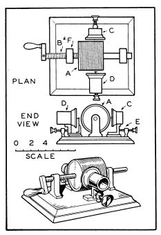
A cardboard pill box or piece of mailing tube may be used to build this recorder. The flaring end can be built up with wood or putty, then fashioned to shape.
