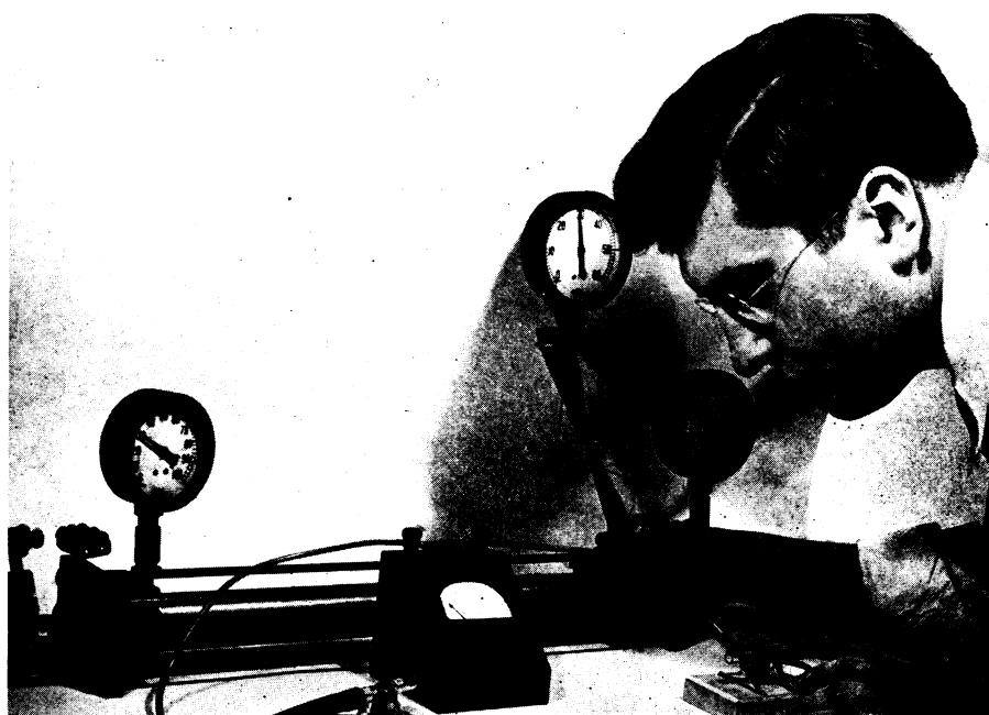
HOT-COLD PIPE —This tube separates hot and cold air. Compressed air is whirled by a steel spiral to make the difference in temperature.
