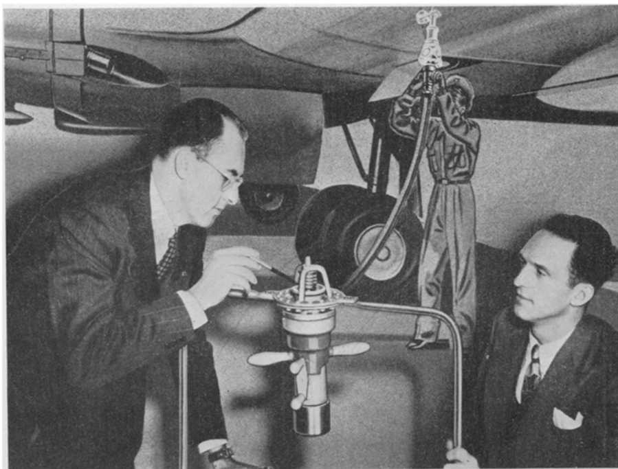
REFUELING VALVE —Underwing valve cuts down refueling delays.
