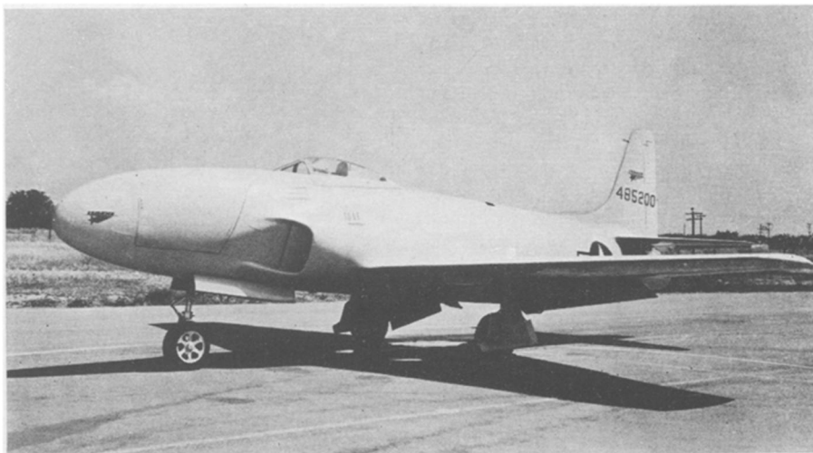
SPEEDY PLANE —The world's speed record is held by this P-80R, a special version of the Army's noted jet-propelled Shooting Star. Leading wing edges are sharper, pilot canopy is lower, and air intakes are redesigned to lessen drag.
