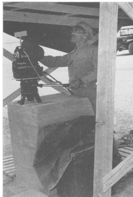
TIMING CAMERAS —Electrically operated, this camera that timed the speed-champion Lockheed P-80R is accurate to 1/1000 of a second.
