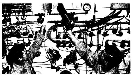
CHECKING RADIATION—Fission product materials emitting high levels of radiation are processed inside a thick walled concrete cell. This shows apparatus on the outside wall where all operations are performed by remote control. Radiation emitted through an opening is being checked with an instrument called a "cutie pie."
