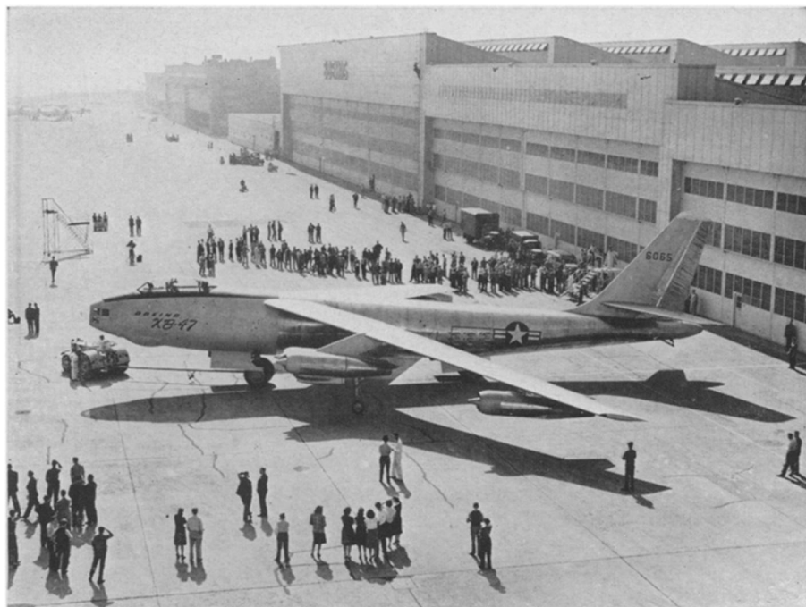
"STRATOJET" —This is the new experimental Boeing XB-47 with six jet engines. Notice the very thin swept back wings, which it is hoped will give the plane great speed, and the position of two of the jets near the wing tips.
