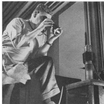
MELTED BY RADIO —The investigator shown is measuring the temperature of thorium with a pyrometer while radio waves bombard it in a tubular high frequency melting chamber of the Westinghouse Lamp Research Laboratories. Thorium powder fuses at 3,600 degrees Fahrenheit.
