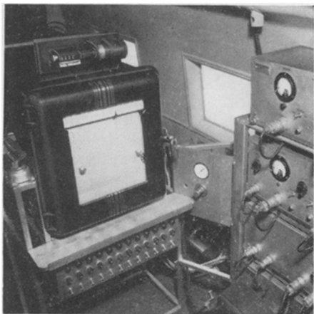
Speedomax instrument in an airplane, recording variations in the earth's magnetic field.
